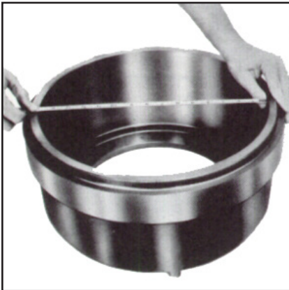
Diameter brake surface (allow for drum wear)
