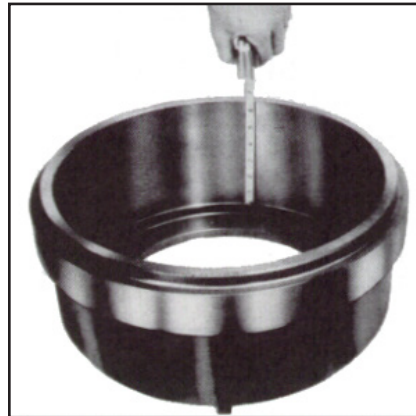
Width of braking surface
